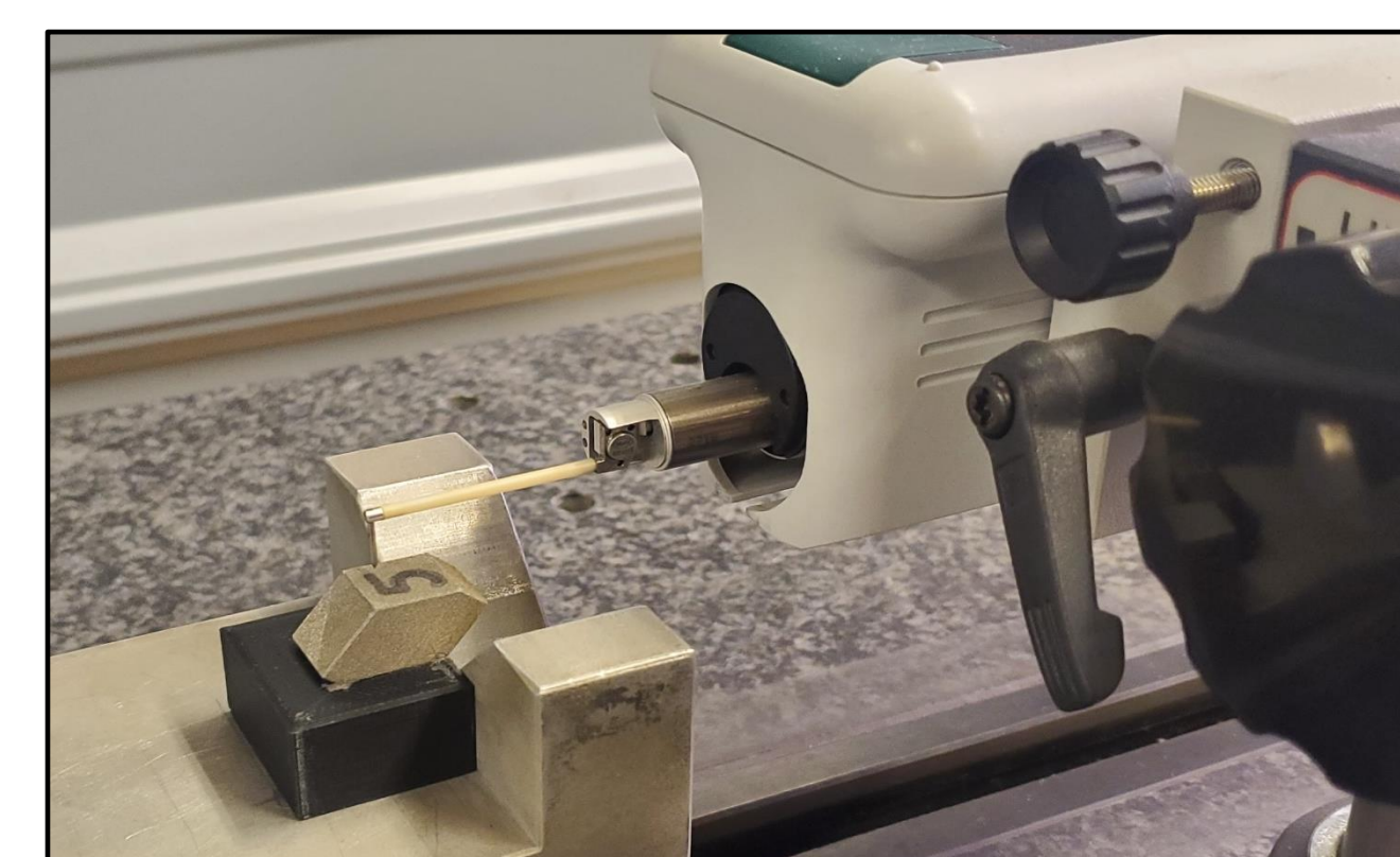
Roughness Data Collection Set-up
